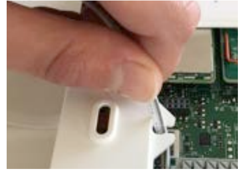
Insert the wire into the strain-relief
