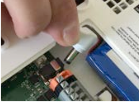
Plug in the power connector
