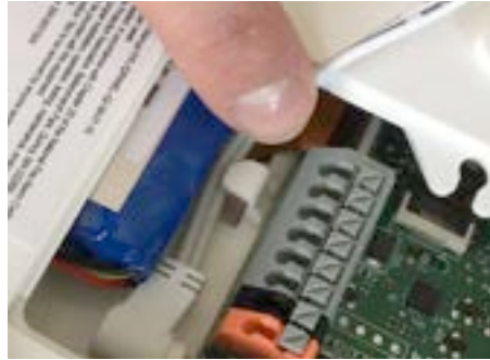
Route the wire behind the retainer clip
